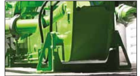
Boom Section Feets prevents from scratch and corrosion
